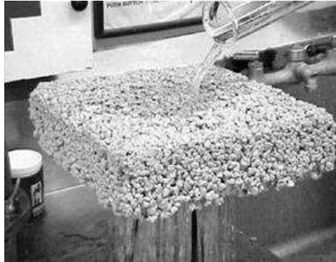
Pervious concrete permits storm water to percolate
