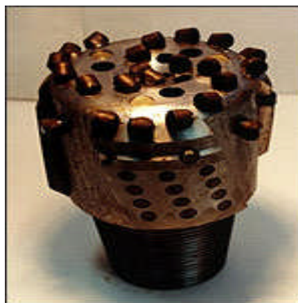
A diamond-studded drill bit developed at Sandia National Laboratories.
